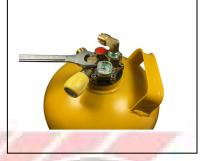
Remove the solenoid blanking cap with a spanner being careful not to damage the plastic contents gauge.
