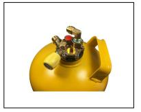
Remove the multivalve contents gauge using a 1.5mm Allen key.
