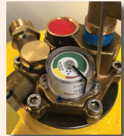
Remove the standard multivalve gauge...
